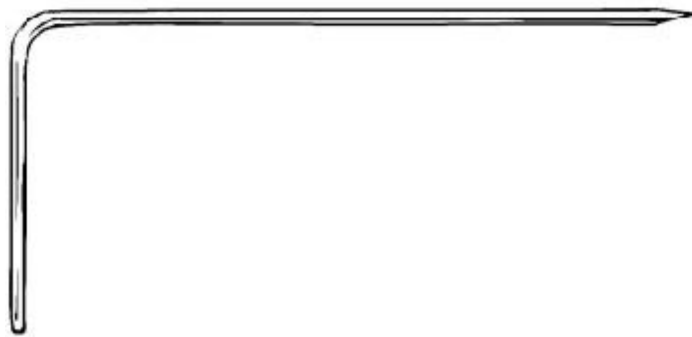
The strong wire must also be sharply pointed
