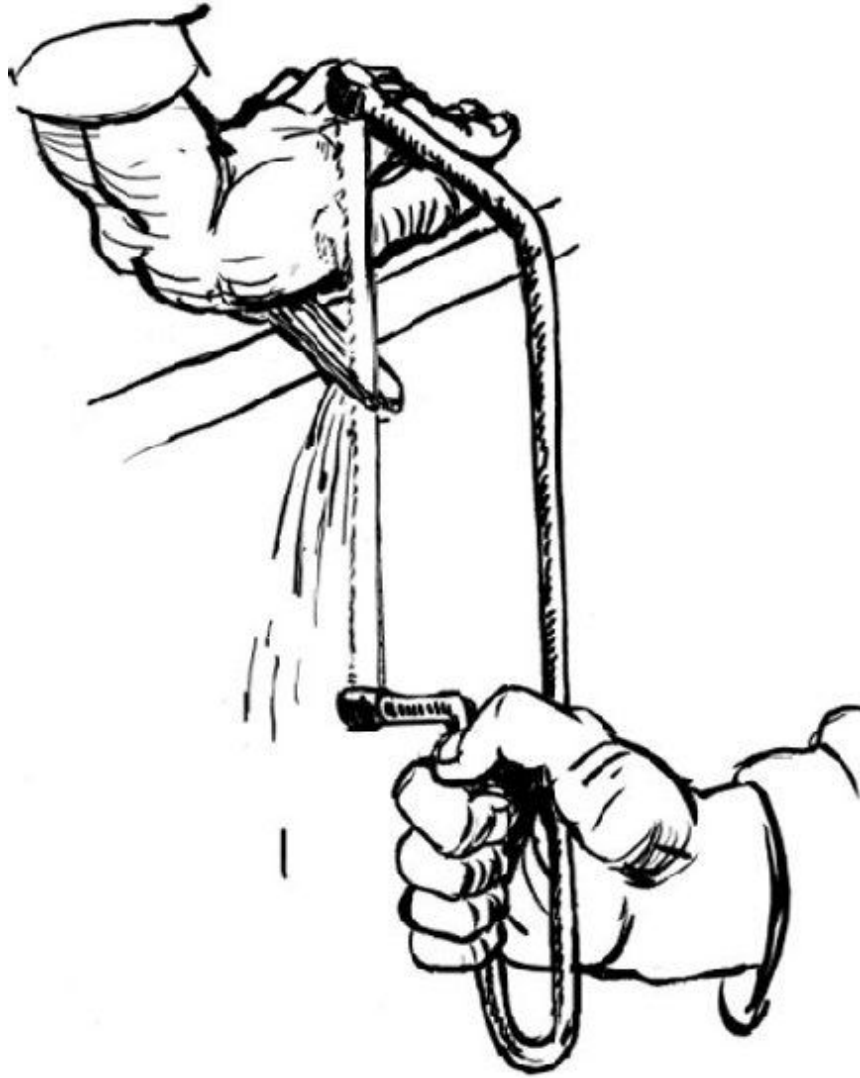
Careful sawing of the key along the first groove
